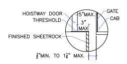
DOOR SILLS TO BE INSTALLED BY GC AFTER THE LIFT SUPPLIER HAS INSTALLED A RUNNING PLATFORM. SILL MUST BE BROUGHT OUT TO NOT LESS THAN ½" AND NOT MORE THAN 1 ¼" TO THE RUNNUNG PLATFORM WHILE MAINTAINING A DISTANCE OF 3" FROM THE HOISTWAY FACE OF THE LANDING DOOR (OR GATE) TO THE HOISTWAY EDGE OF THE LANDING SILL.
