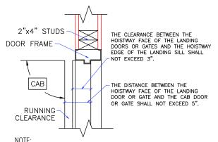
\* FRAMING ON DOOR SIDE OF HOISTWAY MUST BE OF 2x4 CONSTRUCTION TO APPLY TO 5-3 RULE OF ANSI 17.1 CODE.
