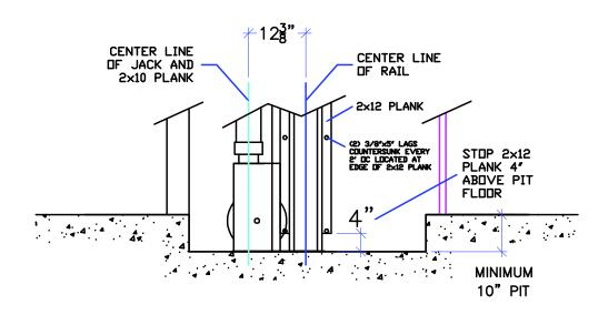
6" MINIMUM 3000 PSI REINFORCED CONCRETE #4 AT 12" O.C. EACH WAY.
