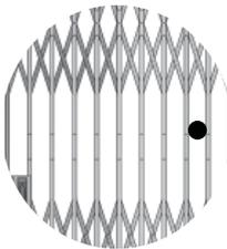
A 3" ball in diameter can NOT fit through anywhere within the gate.
