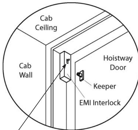
Push the Release Pin Upward
