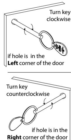
If your elevator is equipped with a GAL "N" Type Interlock, use the key provided to open the lock from outside of the hoistway. Insert the emergency release key into the hole (near the top of the door) and turn (toward the center of the door) to release the interlock while opening the door.
