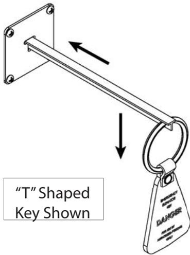
If your elevator is equipped with an Electromechanical Interlock (EMI) use the key provided to open the lock from the outside of the hoistway. To open the door insert the key through the hole in the hoistway door until key stops or the handle contacts the door. If unable to perform this procedure proceed to the instructions for unlocking the door from the inside of the car. GENTLY pry the outboard end of the key to lift the interlock pin. Slowly open hoistway door with interlock pin raised.
