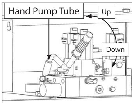
If you are unable to move the elevator to a floor, you can manually raise the car by using the hand pump.
